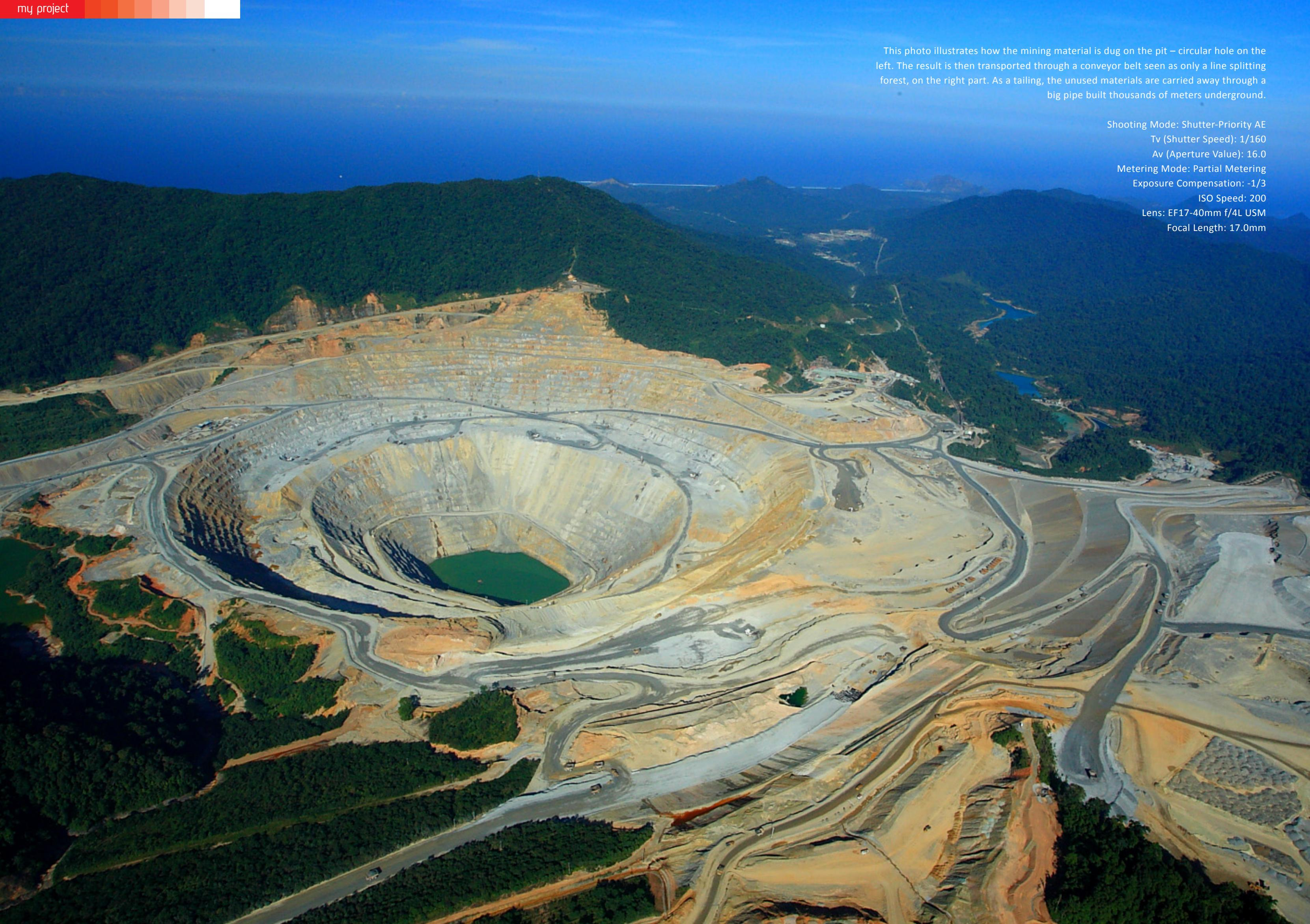
This photo illustrates how the mining material is dug on the pit – circular hole on the left. The result is then transported through a conveyor belt seen as only a line splitting forest, on the right part. As a tailing, the unused materials are carried away through a big pipe built thousands of meters underground.
