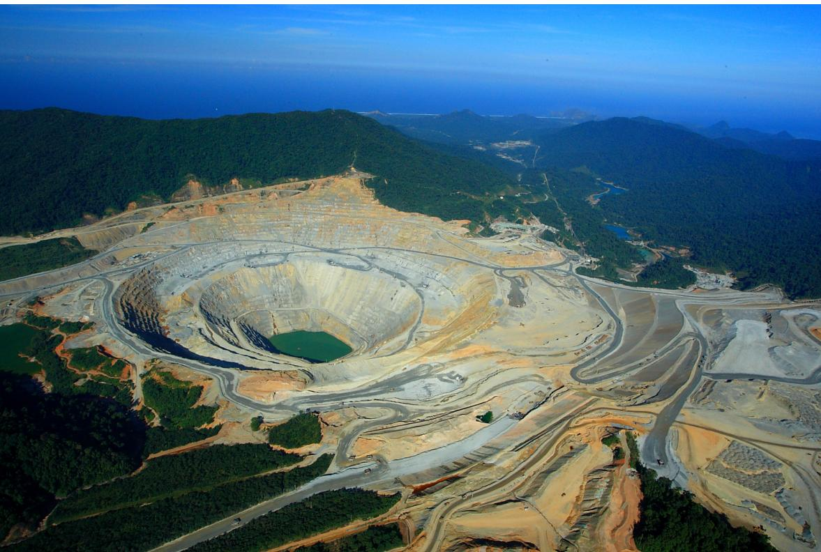
This is the complete site. This photo pictures the mining process; from “pit” peeling on the center right area, to a tailing disposal through pipes heading the open sea on the top right.
